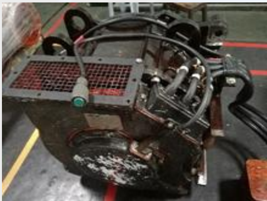
KTMB Class 29 Traction Motor (345kW)
