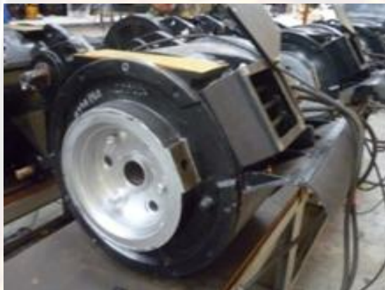
KTMB Class 81 Traction Motor (161kW)
