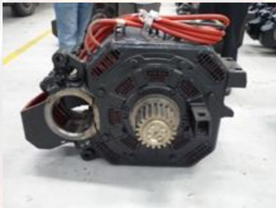
KTMB Class 24 Traction Motor (217kW)
