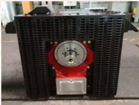
KTMB Class 92 Traction Motor (160kW)
