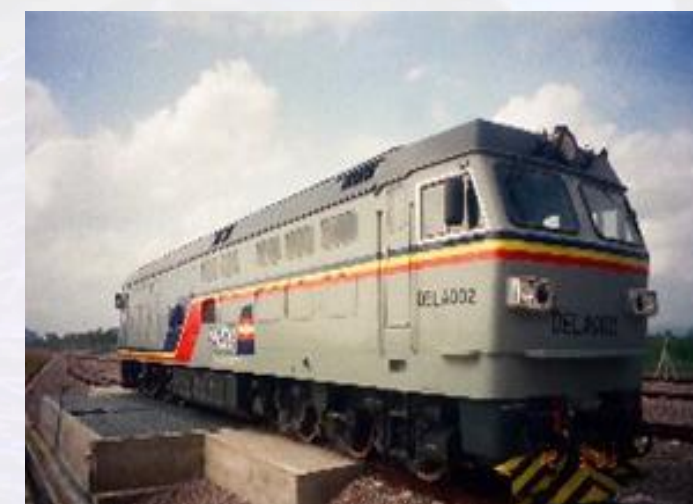
Mainline Diesel Electric Locomotive
