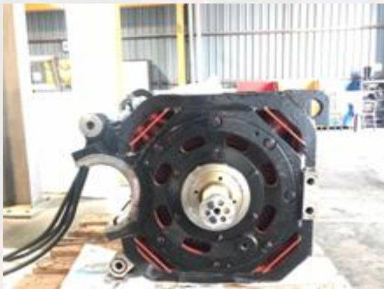
Cambodia Locomotive Traction Motor 1 (165kW)
