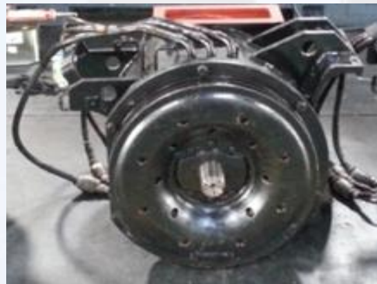
KTMB Class 83 Traction Motor (150kW)
