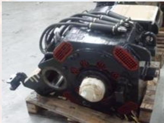
KTMB Class 25 Traction Motor (160kW)
