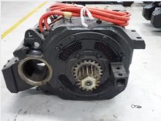
KTMB Class 23 Traction Motor (230kW)
