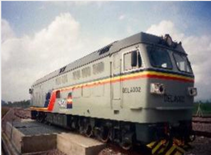
Mainline Diesel Electric Locomotive
