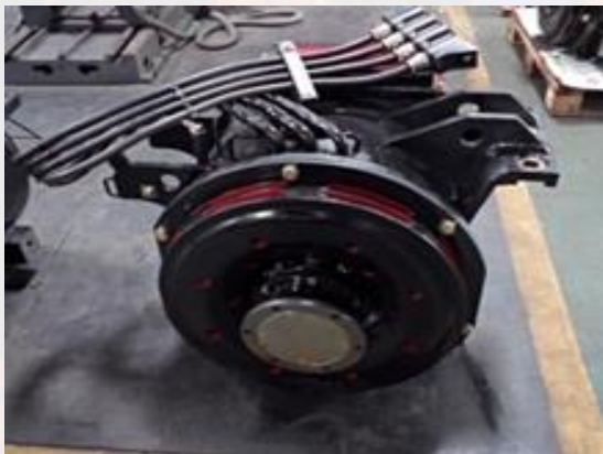
KTMB Class 91 Traction Motor (150kW)
