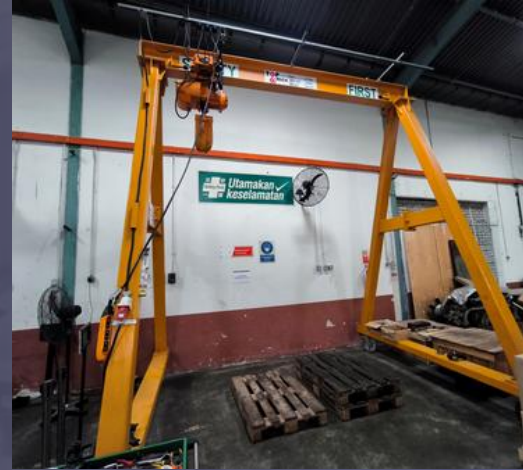
2-Tonnes Portable Gantry Crane
